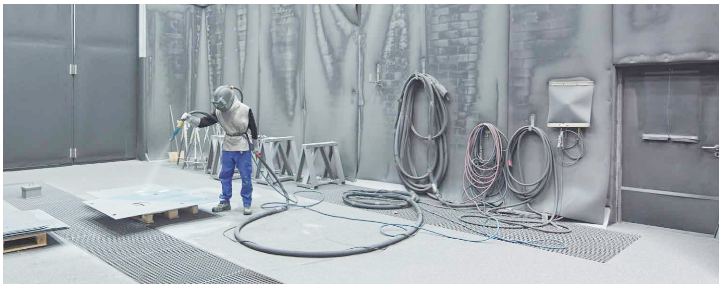
Surface protection work in a blasting hall
